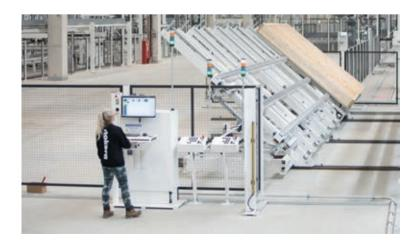
Serial production of a timber module in a NOKERA factory.
